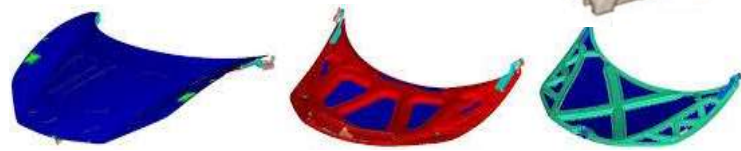
(a) Initial shape (b) Optimal surface (by Out-of-plane variation) (c) Optimal boundary (by In-plane variation)
